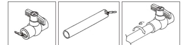
1. Apply sufficient cement on the inner wall of valve and outside wall of pipe, please do not apply too much cement, for it may obstruct the fluid flowing in the valve.
